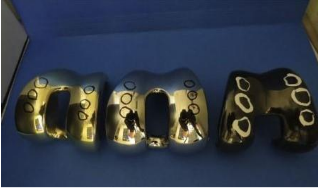
Figure 2-1. Damaged Areas Shown on ZrN-, CoCr-, and Oxinium-Bearing Surfaces Left to Right: ZrN-Bearing Surface, CoCr-Bearing Surface, and Oxinium-Bearing Surface
